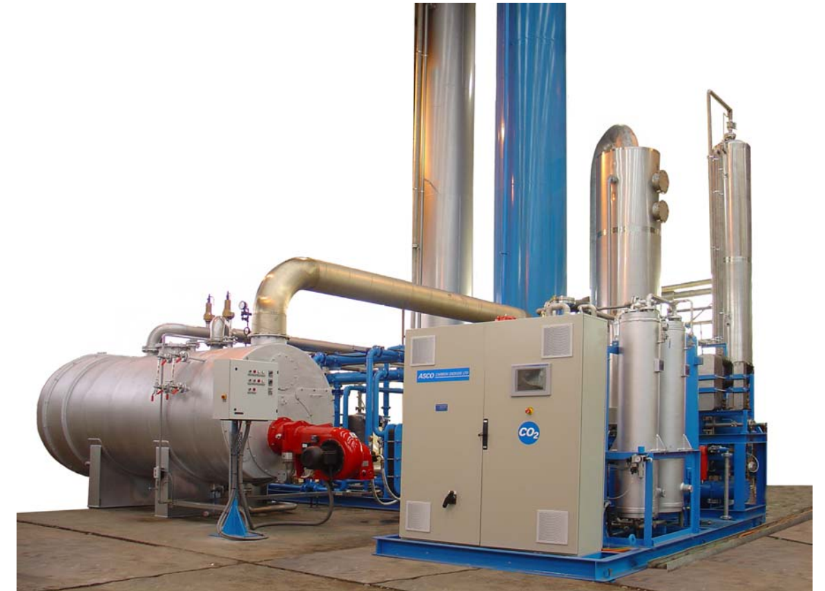
HPA (High Performance Automatic) 500 kg/hr CO2 Production Plant during test at ASCO factory
